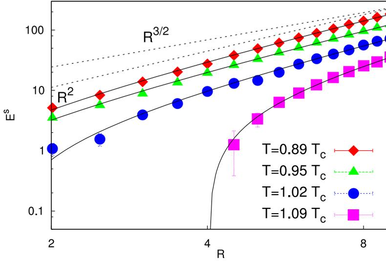
**Figure 2.**  $E^s$  versus excitation radius  $R$  at various temperatures. Full lines are fits using equation (1), with  $\theta = 2$  and  $\omega = 1.5$ . Dotted lines show the power laws with exponents 2 and 3/2 for reference. Error bars are smaller than symbol size.
